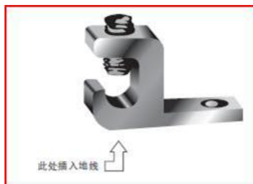
Figure 5 Schematic drawing for PV module grounding
